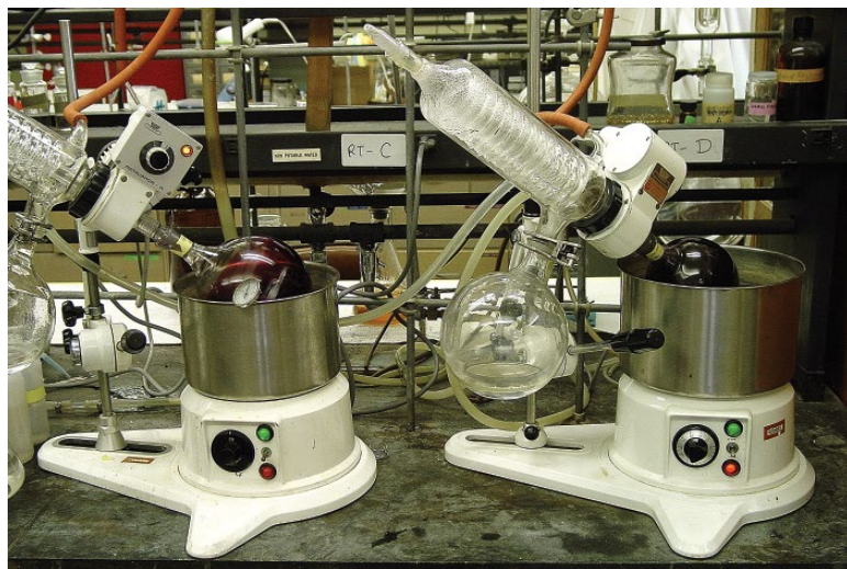
Figure 2.9 Rotary evaporators are used to remove solvents from plant extracts. The extract is heated under vacuum; volatile solvents condense on chilled coils and drip into a collection flask.
