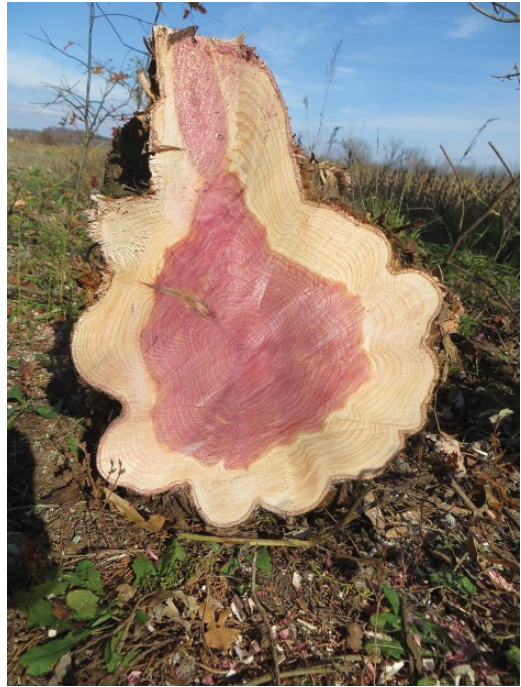
Figure 1.69 Cross section of red cedar ( Juniperus virginiana L.) showing the vibrant red heartwood and lighter sapwood. According to the growth rings, this tree was 35 years old.
