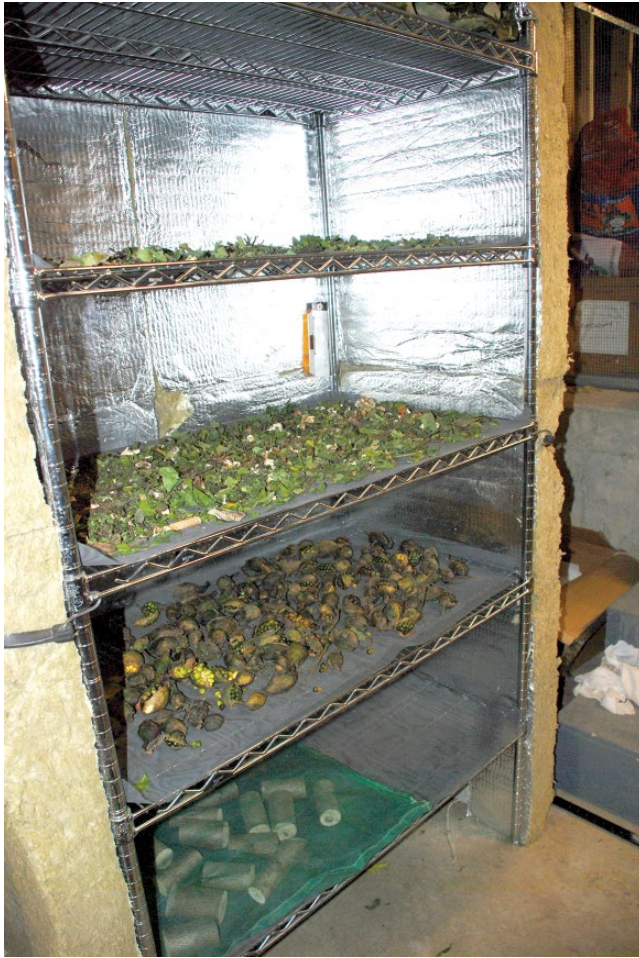
Figure 1.79 Plant material drying in a forced air drier at the New York Botanical Garden Herbarium.
