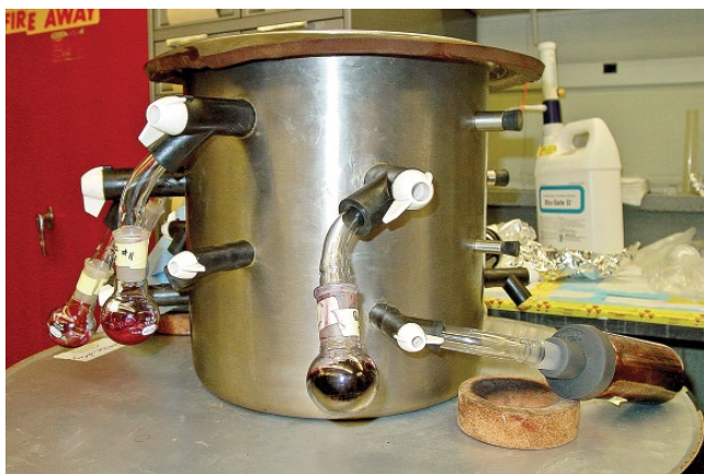
Figure 2.10 Example of a drum manifold lyophilizer. After solvents are removed, plant extracts are frozen in round-bottomed flasks, and then placed on the lyophilizer until water is removed via sublimation.
